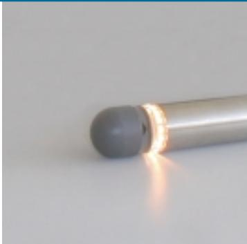
The tool generates a continuous oriented 360° image of the borehole wall using an optical imaging system. (downhole CCD camera which views a image of the borehole wall in a prism). The tool includes a orientation device consisting of a precision 3 axis magnetometer and 3 accelerometers thus allowing accurate borehole deviation data to be obtained during the same logging run (accurate and precise orientation of the image).
