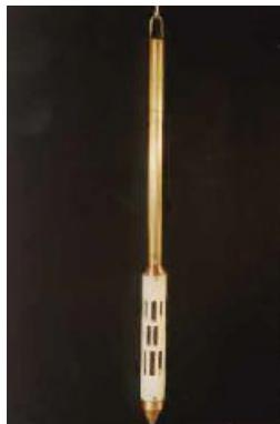
To generate the sparker pulses within the borehole the p-wave sparker probe **SBS 42** is used (left). The SBS 42 consists of a probe tube and a rubber tube system. The sparker predominantly produces high frequency p-waves even over large distances as shown below.
