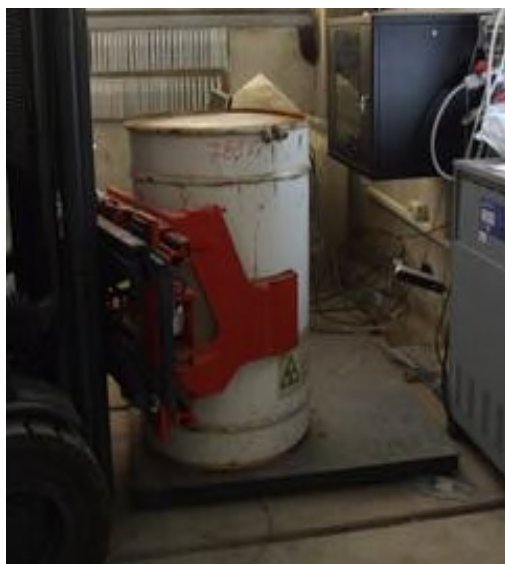
Prelevamento overpack e pesatura overpack
