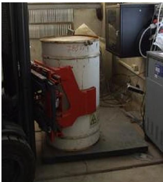
Prelevamento overpack e pesatura overpack
