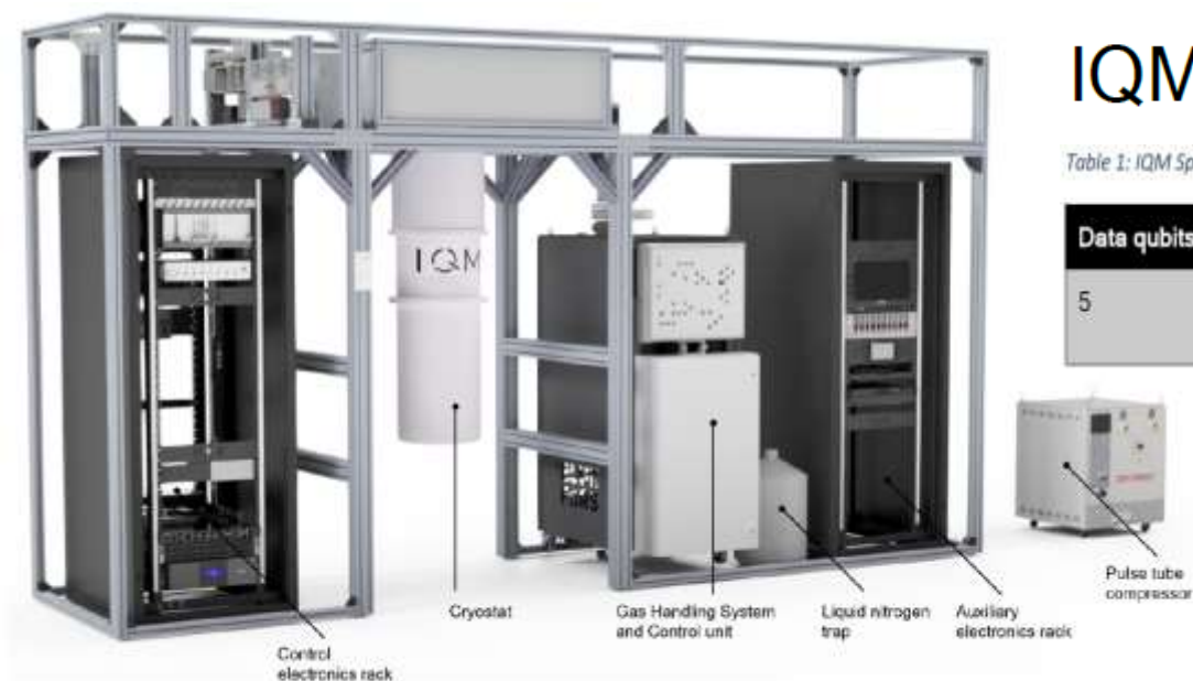
Figure 2: Physical parts and layout of IQM Spark™ quantum computer. System covers are not shown. Image is representative only and subject to change.
