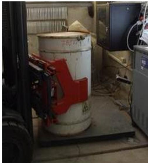
Prelevamento overpack e pesatura overpack
