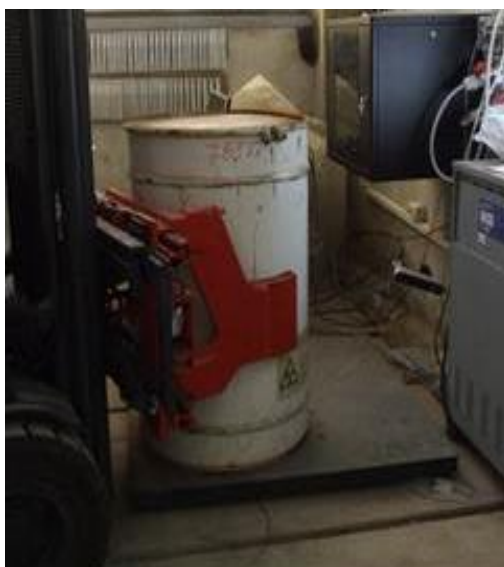
Prelevamento overpack e pesatura overpack
