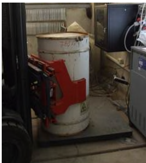
Prelevamento overpack e pesatura overpack
