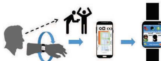
Figure 1-7: How HANGER works
